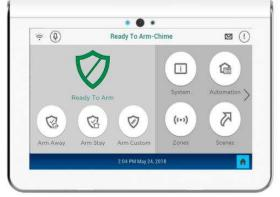
Wireless Security Control with self-contained **Digital Communicator and battery backup**
